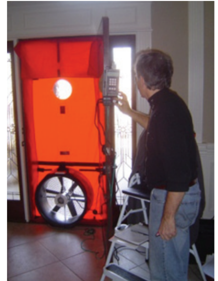
Figure 17: Blower door testing
