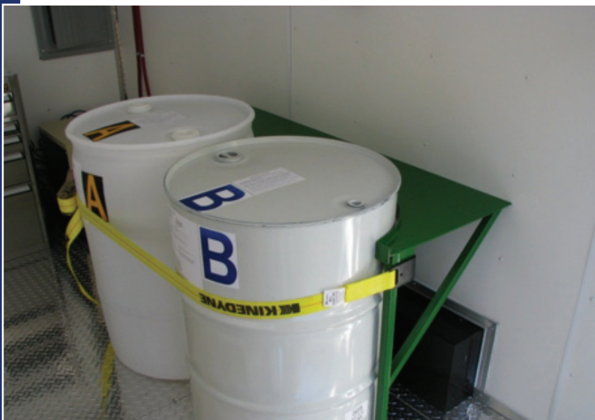
Figure 1: Drums strapped inside truck
