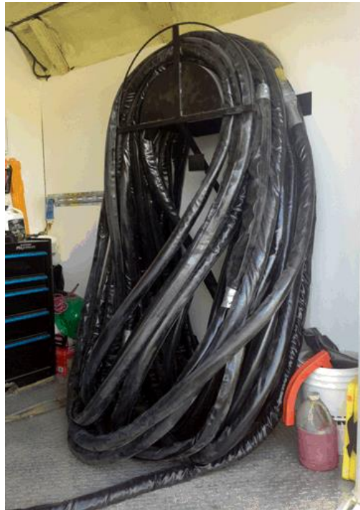
Figure 14 - Standard rack design which stacks more than one layer of hose. This hose must be removed from the rack down to a single layer before preheating.
