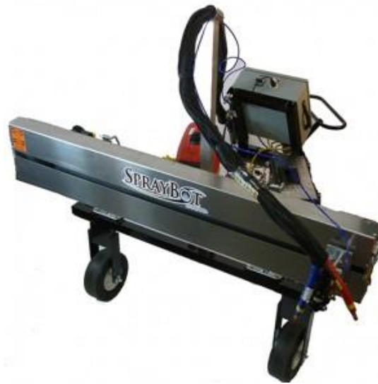
Figure 26 – Robotic Spray System for Roofing Applications
