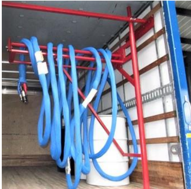
Figure 16 - 180-degree swing-out rack releases the hose directly out the rear door of the rig.
