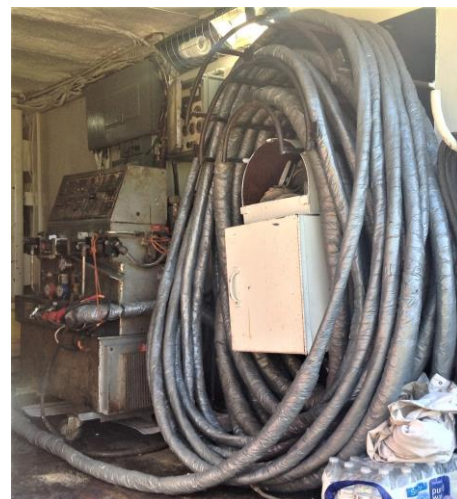
Figure 15 - Three-tiered rack hangs the hose in single layers, preventing electromagnetic effect and overheating of the hoses, enabling preheating of the entire hose while on the rack.
